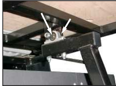
Lifting Arm shown under table top (one at each end of the table)
